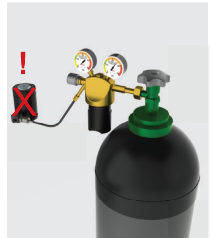
When charging, ensure piston rod is fully extended. Maximum Charge pressure must not be exceeded.
